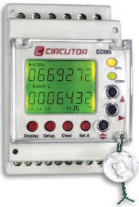
The **EDMk** three-phase electronic energy meter is capable of measuring consumed and generated energy (four quadrants): Active energy (consumed and generated), inductive reactive energy (consumed and generated) and capacitive reactive energy (consumed and generated), plus metering partial energies.
